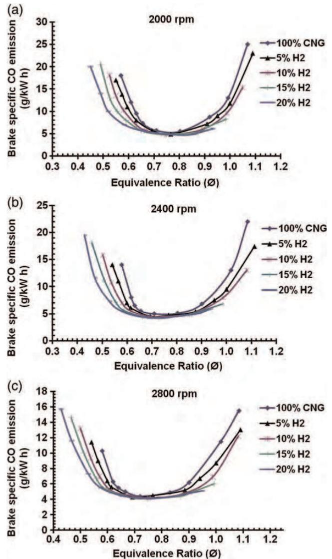
Figure 2. (a–c) Variation of brake-specific CO emissions versus equivalence ratio for various hydrogen blends at 2000, 2400 and 2800 rpm.
