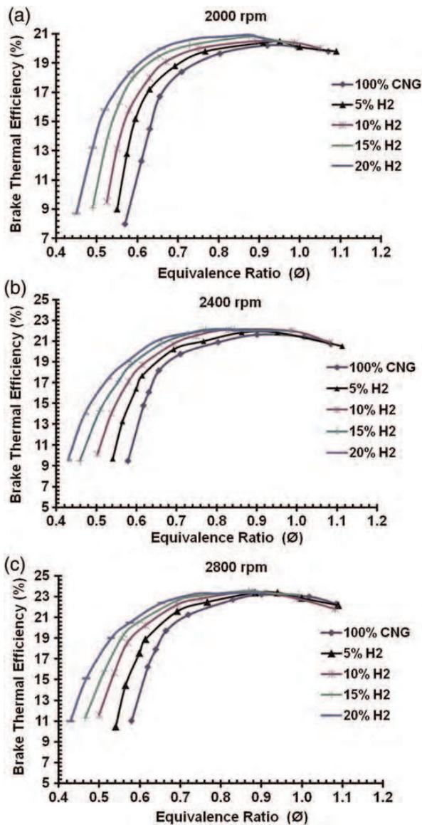
Figure 5. (a–c) Variation of BTE as a function of Equivalence Ratio for various hydrogen blends at constant speed of 2000, 2400 and 2800 rpm.
