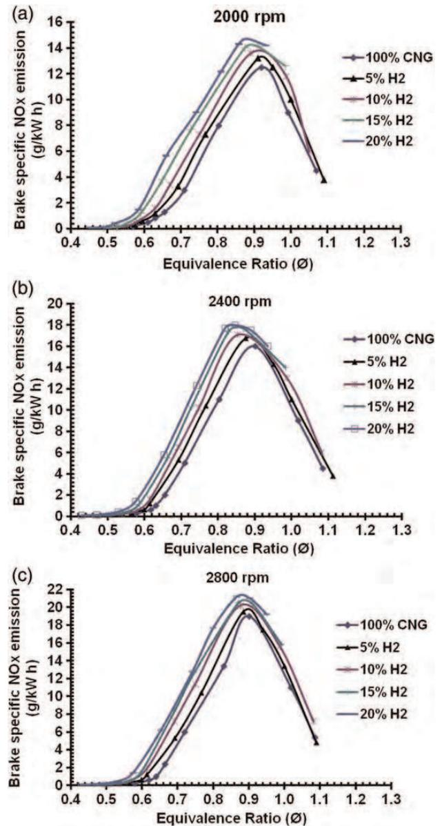
Figure 4. (a–c) Variation of brake-specific NO<sub>x</sub> emissions as a function of equivalence ratio for various hydrogen blends at constant speed of 2000, 2400 and 2800 rpm.
