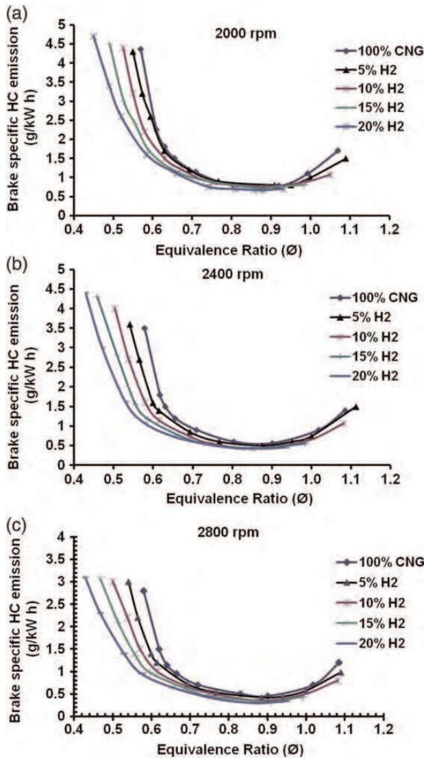
Figure 3. (a–c) Variation of brake-specific HC emissions versus equivalence ratio for various hydrogen blends at constant speed of 2000, 2400 and 2800 rpm.
