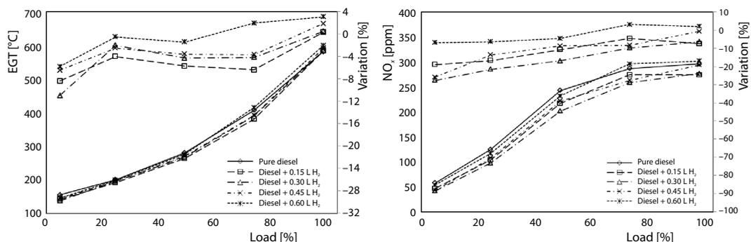
Figure 4. Variation of EGT (a), and NO<sub>x</sub> emissions (b)
