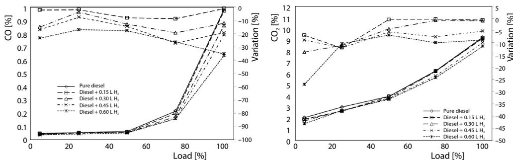
**Figure 6. Variation of CO (a) and CO<sub>2</sub> (b) emissions**
