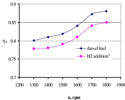
Fig. 11 Volumetric efficiency
