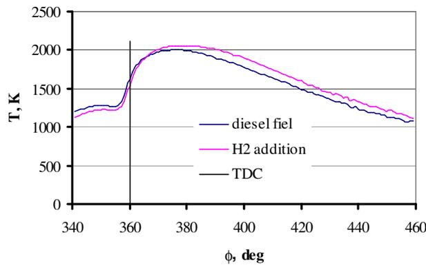
Fig. 6 Cylinder temperature
