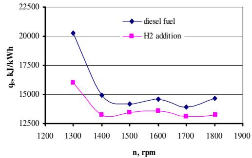
Fig. 8 Brake specific heat consumption
