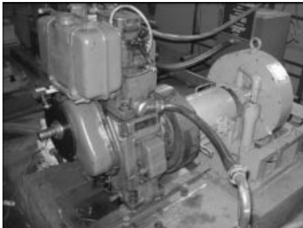
Fig 6. Single cylinder kirloskar taf-1
