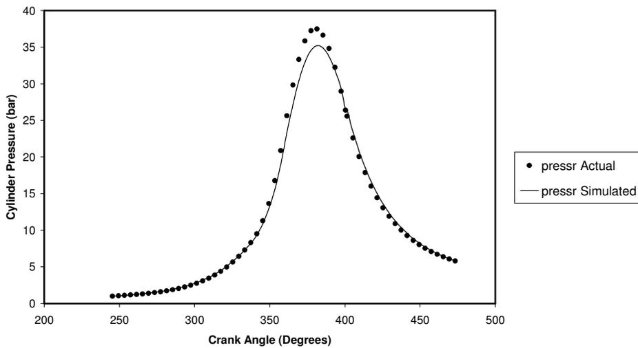
Figure 1-B. Pressure-Crank Angle comparison the experimental & theoretical results
