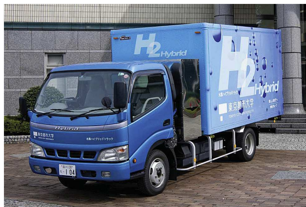
Fig. 3 – Hybrid light duty truck equipped with a 4 L 91 kW hydrogen engine, demonstrated by Tokyo City University [3]. Permission to reproduce granted by copyright holder Tokyo City University.
