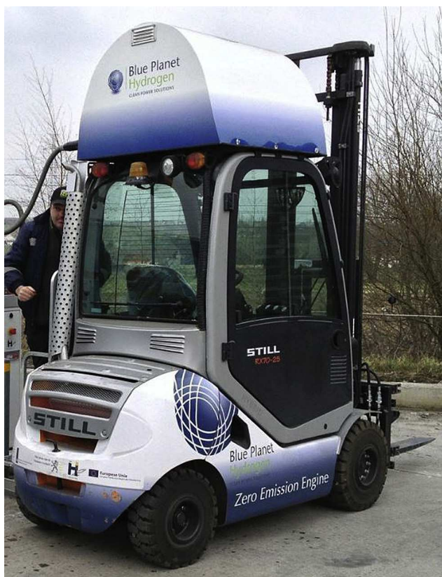
Fig. 2 – Forklift truck equipped with a H 2 ICE, part of the demonstration activities within the Hydrogen Region Flanders – South-Netherlands project [21].
