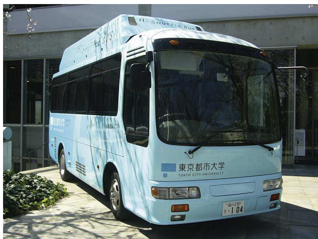
Fig. 4 – Microbus equipped with a 4.7 L 105 kW hydrogen engine, demonstrated by Tokyo City University [3]. Permission to reproduce granted by copyright holder Tokyo City University.
