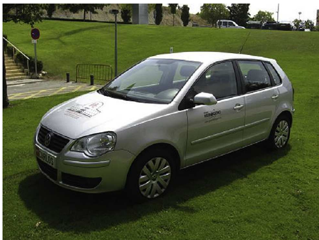
Fig. 1 – Bi-fuel (gasoline/hydrogen) VW Polo demonstrated by the University of Navarre [5]. Copyright 2012, Elsevier, reprinted with permission.
