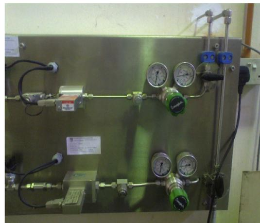
**Fig. 4 – High pressure regulator panel.**
