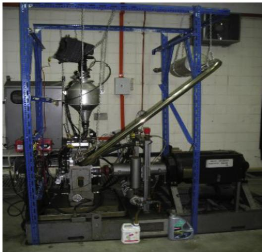
**Fig. 3 – The engine test-bed.**
