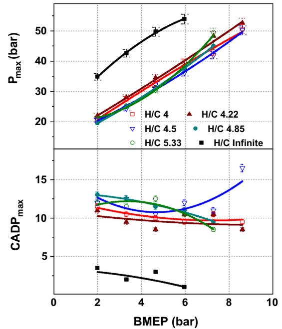
Fig. 3. Variation of peak in-cylinder pressure and its location.
