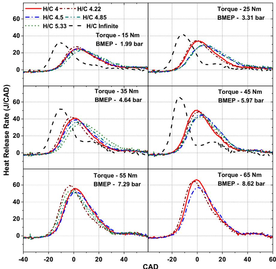
Fig. 4. Variation in heat release rate for HCNG test fuels.
