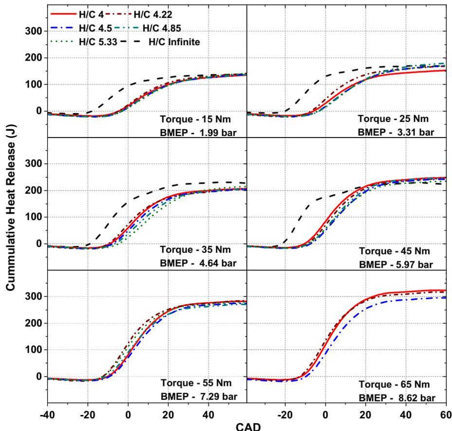
Fig. 5. Variation in cumulative heat release for HCNG test fuels.
