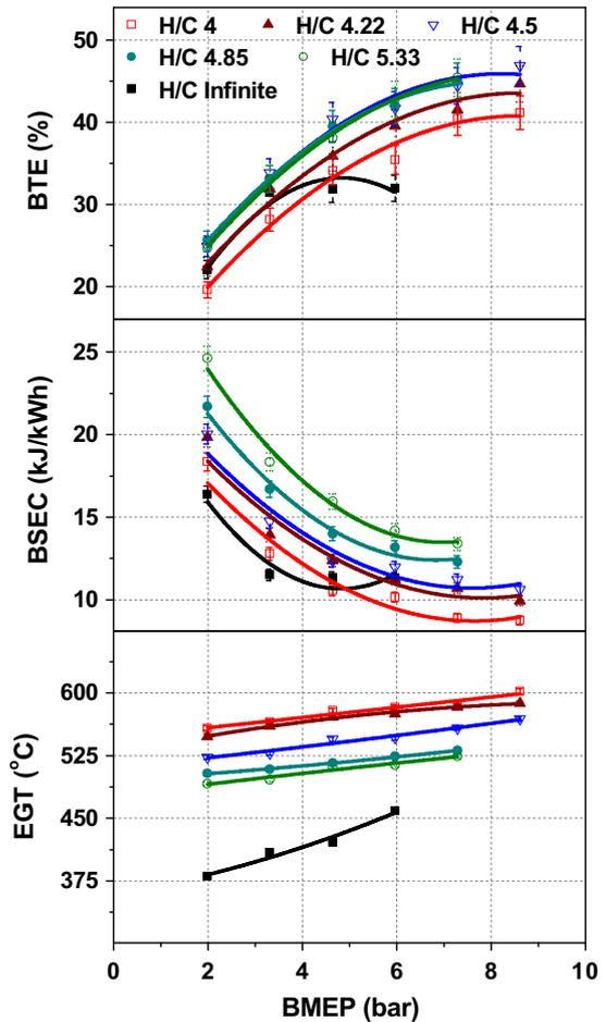
Fig. 8. Variations in brake thermal efficiency, brake specific energy consumption, and exhaust gas temperature for HCNG test fuels.
