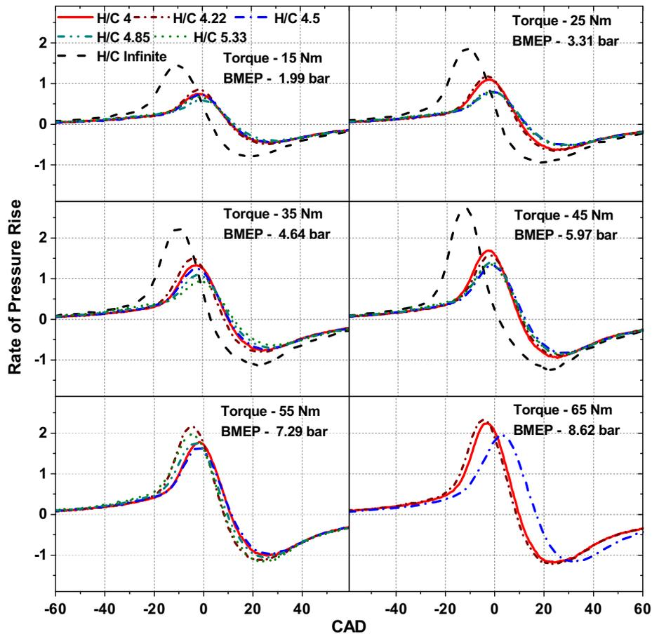
Fig. 6. Variation in rate of pressure rise for HCNG test fuels.
