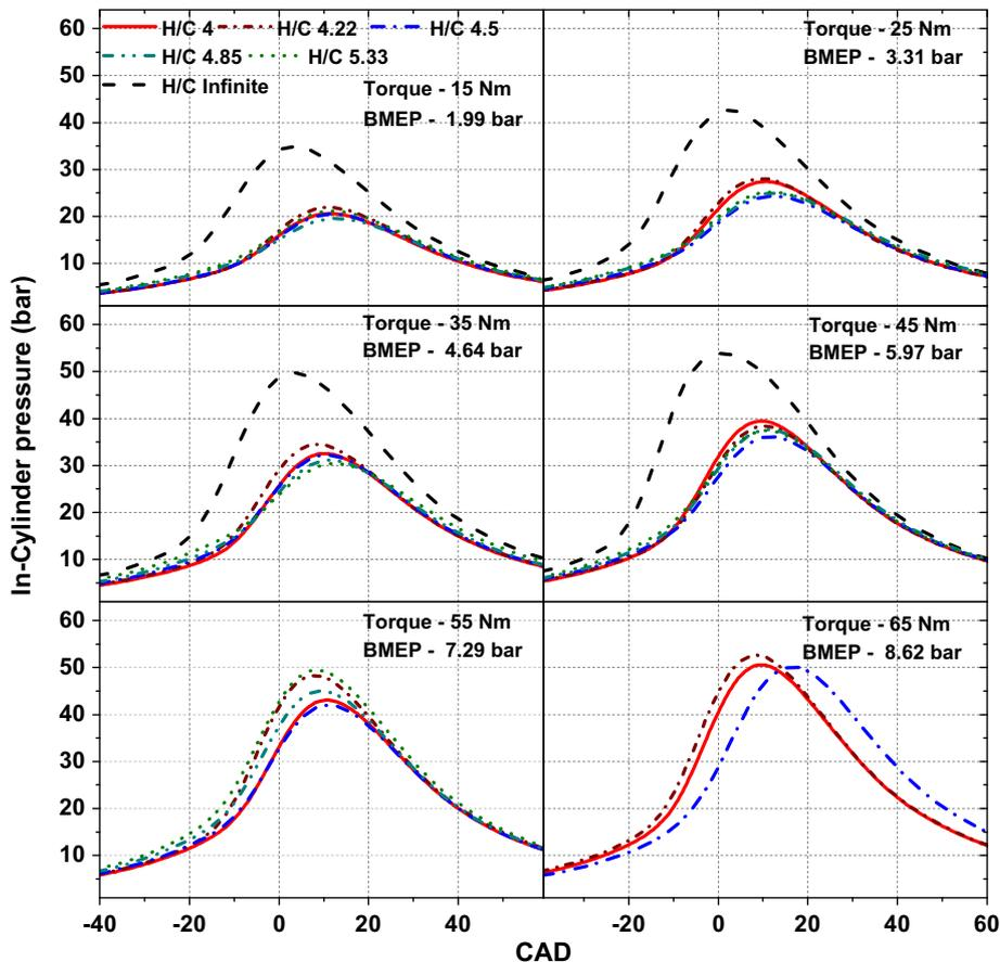
Fig. 2. Variation of in-cylinder pressure for HCNG test fuels.
