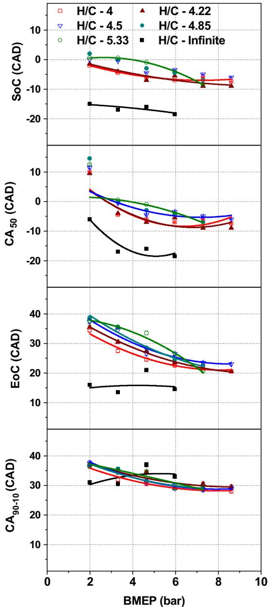
Fig. 7. Variation of start of combustion, combustion phasing, end of combustion and combustion duration for HCNG test fuels.
