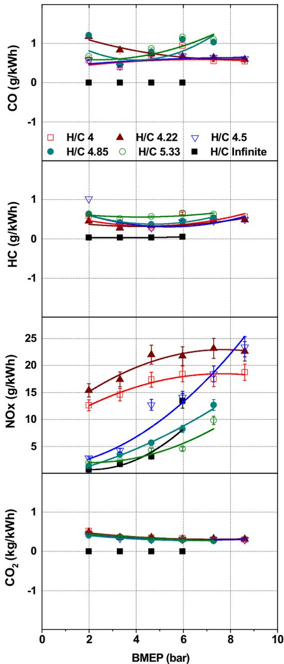
Fig. 9. Variations in CO, HC, NOx and CO<sub>2</sub> emissions.
