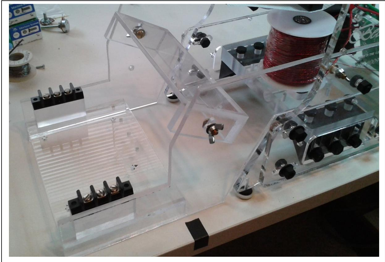
The frame extension pieces bolt to the vertical supports of the original SG frame using one large black nylon nut and bolt which is also reinforced by the addition of two brass bolts and wing-nuts. The shape of the clear acrylic extension pieces is shown here, outlined by the **GREEN** line.
