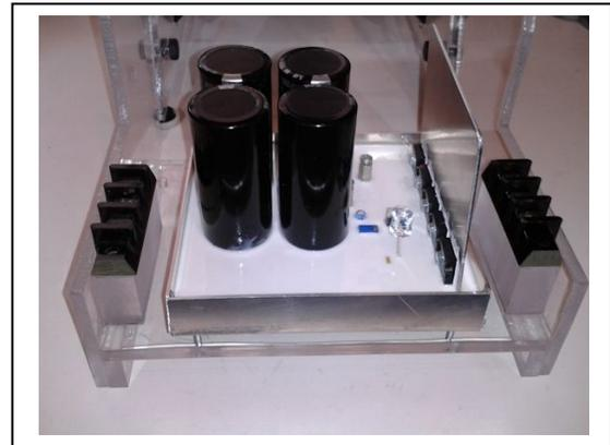
Two terminal blocks were mounted, one on either side of the capacitor module, to lead to external wiring of the system.
