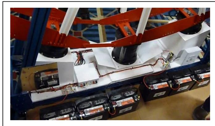
The input was 36 volts (three 12 volt batteries in series) and the output was the same. The batteries boiled continuously during operation, and John never ran it for more than 30 minutes at a time in full power mode. The batteries were too small to be charged that hard.
