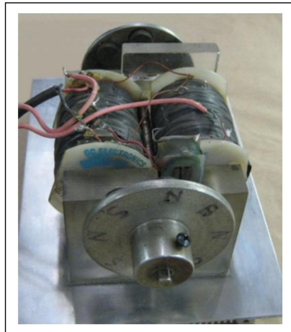
For this type of operation, Ron needed a double-sided switching circuit, so the coils could be energized and then completely disconnected from the supply before being reconnected in the opposite polarity.
