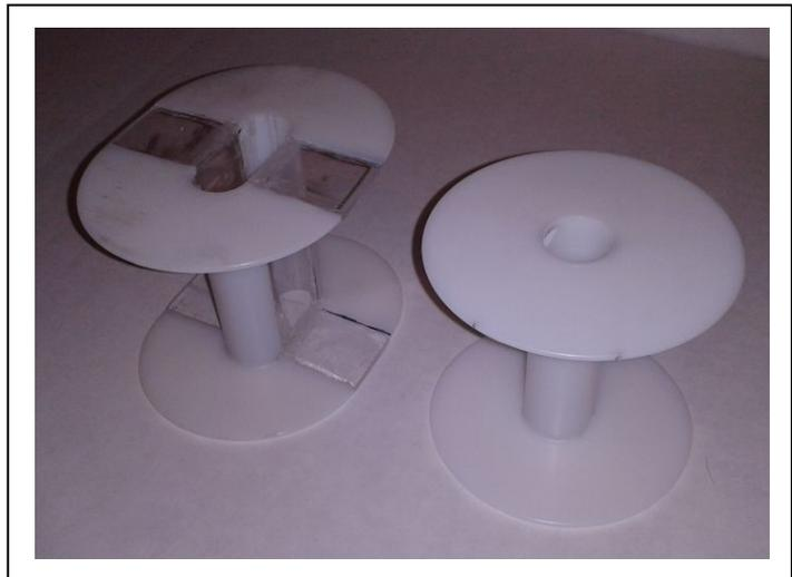
Therefore, a plastic spool like the one used for the power coil was cut in half and the center section was extended by 1 inch.
